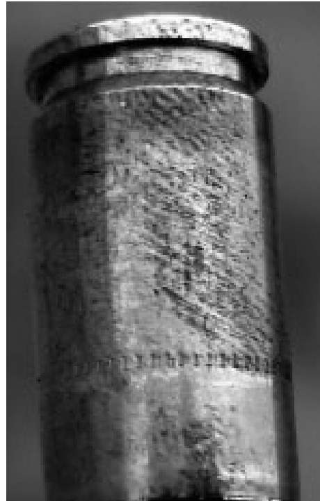
FIG. 24—Ridge detail development for fingerprint deposited on brass 9 mm pistol cartridge shown in Fig. 13 after electrostatic enhancement.
